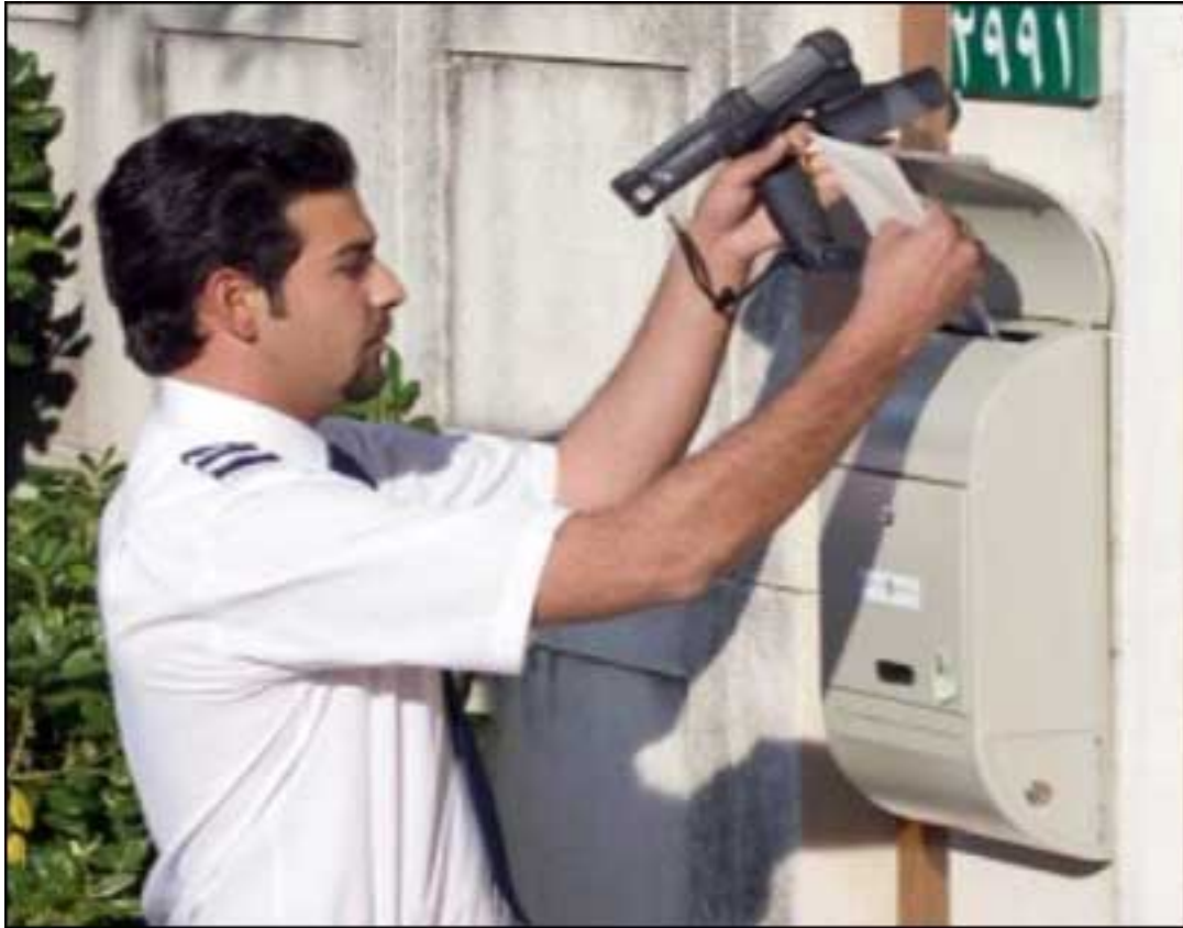
Saudi postal carriers use handheld RFID interrogators to identify the mailboxes before slipping letters into them.
