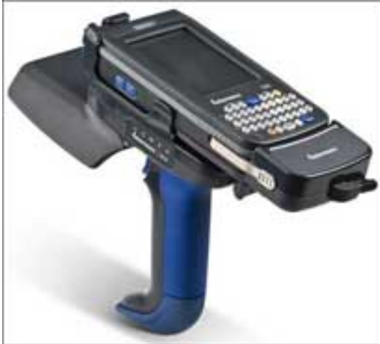
The Intermec CN3 mobile computer and add-on IP30 RFID interrogator
